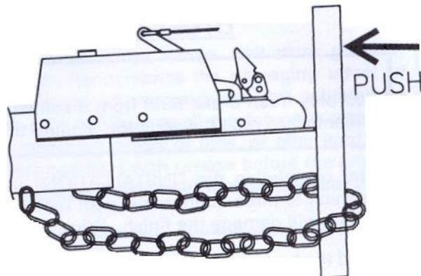
3. Hook the trailer's safety chains (**NOT** the actuator's break-away cable/chain) together to form a loop, which is centered below the actuator's coupler as shown in the figure above.
